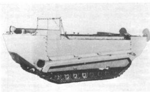
Carrier, Cargo, Amphibian, M29C (Studebaker 'Water Weasel') 6-cyl., 65 bhp, 3F1R×2 (2-speed final drive at rear), 192×67¼×71(54) in, 4778 lb. 20-in tracks. Ground pressure 1-93 lb/sq in. Water propulsion effected by the tracks. Speed in water approx. 4 mph. Controlled differential.
